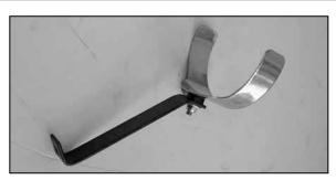
6. On vehicles that come equipped with A/C, assemble the saddle bracket onto bracket (07164A) as shown.
