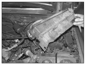
5. Remove the crank case vent from air box then remove the two 8mm bolts that reatin the air box to vehicle. Then remove air box from vehicle as shown.
