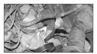
7a. On vehicles that do not come equipped with A/C, mount the saddle bracket assembly from step 6a onto the idler pully bracket as shown. NOTE: Be sure to place the provided spacer (07849) under the bracket.
