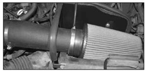
17. Install the air filter onto the new intake tube as shown.
