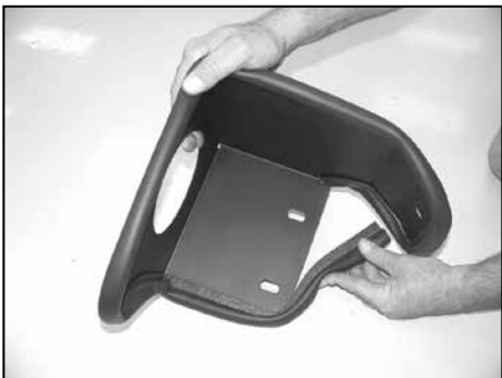
14. Install edge trim onto the heat shield as shown. Trim if needed.
