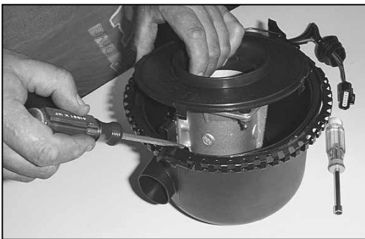
11. Using a flat blade screwdriver, push in and release the four clips that retain the mass air sensor retaining plate.
