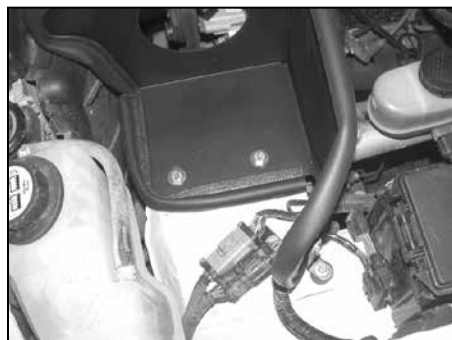
18a. On vehicles not equipped with cruise control, set the heat shield into position on the air filter mounting bracket and then secure the heat shield with the provided hardware as shown. NOTE: The heat shield mounting bracket will be secured to the rubber mounted stud installed in step #15a.
