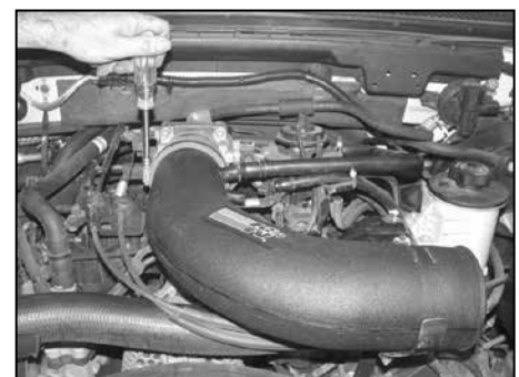
24. Install the K&N® intake tube onto the throttle body and tighten the hose clamp.
