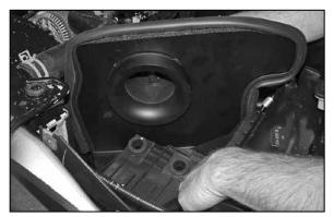
28a. On 2004 and later vehicles, lift up the air boxevap bracket and install the heat shield as shown.
