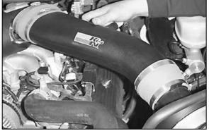
30. Install the intake tube.
