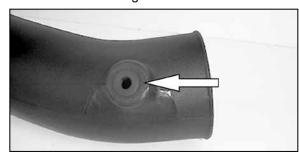
24. On models equipped with an external air temperature sensor, insert the grommet into the hole drilled in the  $K\&N^{\otimes}$  intake tube.
