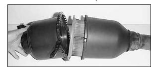
15. Disassemble the air cleaner assembly.
