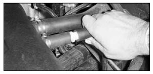
37. Connect the PCV line to the vent hose using the hose mender provided.
