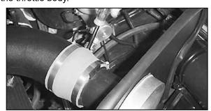
32. Tighten the hose clamp on the stepped hose at the mass air sensor.
