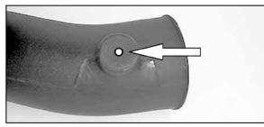
23. On models equipped with an external air temperature sensor, drill out the drill point in the K&N® intake tube using a 11/16" drill bit.
