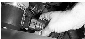
38. Reconnect the primary mass air sensor electrical connection.
