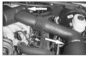
6. Loosen the hose clamps on the intake tube at the air cleaner and throttle body.
