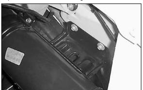
13. Loosen the two bolts that retain the evaporative canister mounting bracket to the inner fender.
