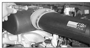
31. Tighten the hose clamp on the hump hose at the throttle body.
