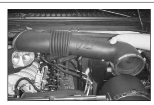
7. Remove the stock intake tube.
