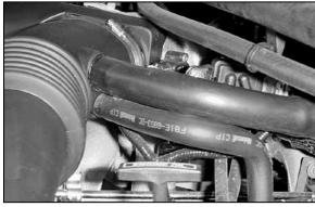
5. Detach the idle air control and PCV lines from the stock intake tube.
