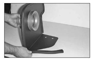
21. Install the trim seal onto the heat shield as shown.
