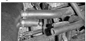
36. Attach the vent hose provided to the small vent fitting on the intake tube.
