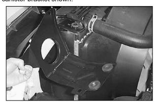
11. Remove the air cleaner mounting bracket. NOTE: On 2004 and later vehicles, this bracket is not removed as it is one piece.
