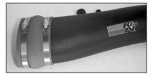
26. Install the hump hose onto the intake tube and tighten the hose clamp.
