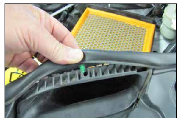
6. Unhook the edge trim from the fresh air intake scoop.
