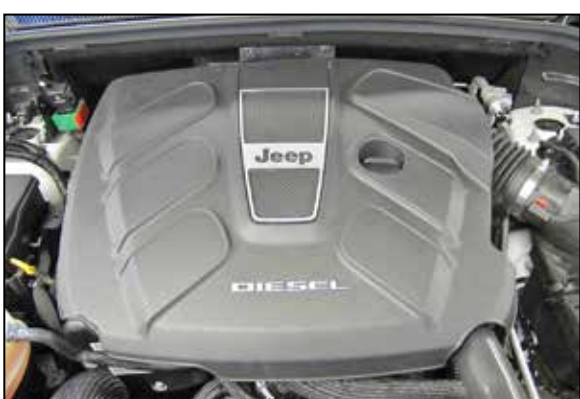
2. Lift up the decorative engine cover and remove it from the engine.
