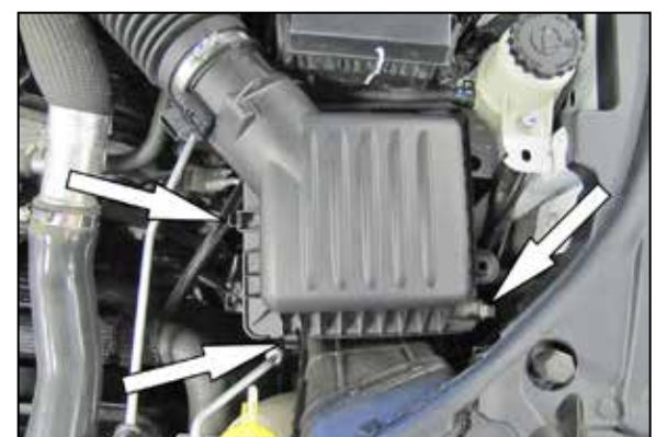
5. Release the three clips securing the upper air filter housing.
