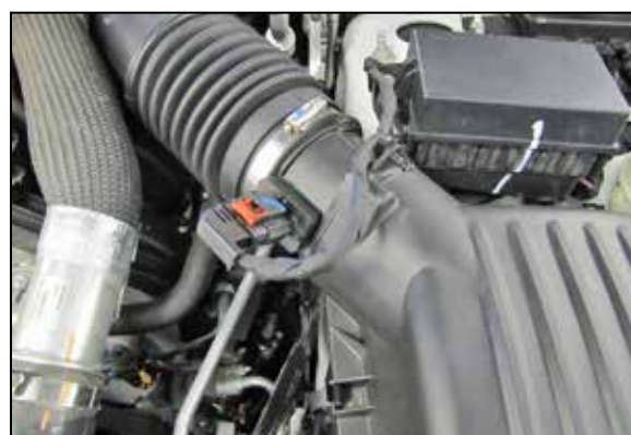
3. Disconnect the mass air sensor electrical connection.
