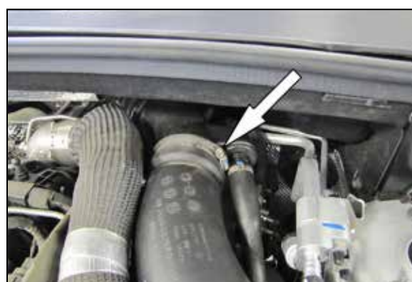
4. Loosen the hose clamp securing the intake tube to the turbo inlet pipe.
