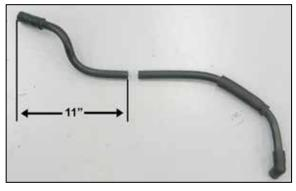
8. Measure 11" from the air filter end of the crank case vent tube and then trim the crank case vent tube as shown.
