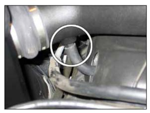
26. Connect the crank case vent hose to the fitting installed into the K&N<sup>®</sup> intake tube and secure with the provided hose clamp.
