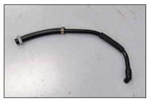
9. Install the provided vent hose onto the cut hose with the provided hose clamps as shown.
