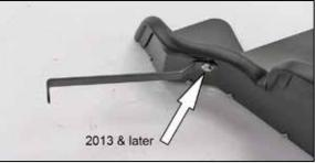
16. Install the heat shield mounting bracket (083103-1A) onto the heat shield using the provided hardware.
