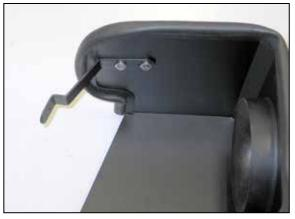
15. Install the heat shield mounting bracket (083127A) onto the heat shield using the provided hardware.
