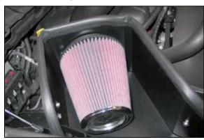
28. Install the K&N® air filter and secure with the provided hose clamp.
