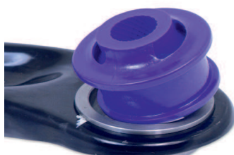
Align slots and push bush into shell
