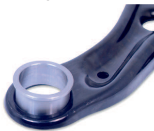
Fit shell in from radius side
