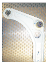
Align score line on bush parallel to inside of wishbone
