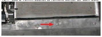
122. Use a 10mm socket to install the heat exchanger, using the 20mm bolts supplied in Bag #2 on the side, and the stock air dam bolt on the bottom.
