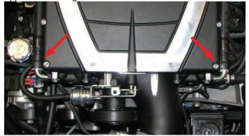
194. Lower supplied air filter onto the radiator shroud.
