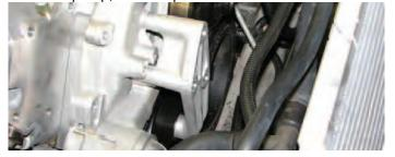
109. Use a 15mm socket and the two stock bolts to mount the new tensioner bracket onto the water pump then torque them to 37 ft-lbs.
