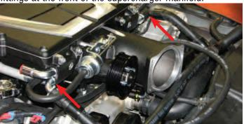
170. Install the passenger side PCV hose on the valve cover fitting by sliding the hose onto the valve cover fitting.
