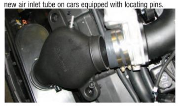
193. Install the hose barb supplied in Bag #5 into the new air inlet tube.
