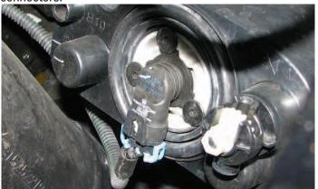
12. Remove four body pins (two on each side) by reaching up through the bottom of the fascia.
