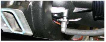
155. Remove the water passage block-off located at the rear of the driver side cylinder head. Grind a 1/4" of material off the inside corner of the block-off at a 45° angle, then reinstall it.
