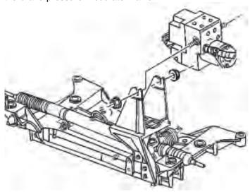
59. Use a 6mm Allen tool to hold the tie rod ball stud stationary while using an 18mm wrench to loosen the nut.
