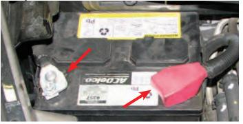
3. Use a 13mm socket and an extension bar to loosen and remove the battery hold down.
