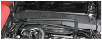
138. Connect the heat exchanger hose assembly to the heat exchanger through the hole drilled in the shroud. Secure the fitting with a hose clamp supplied in Bag #2.
