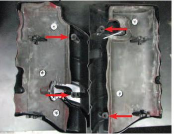
180. Install the stock grommets into the coil cover brackets supplied in Bag #6.
