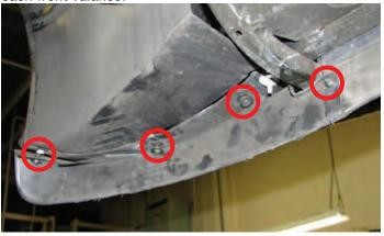
14. The sides of the fascia can be pulled away from the clips holding it in place, then down off the studs. The center section must be pulled up and over the nose section, and the whole assembly pulled straight off and set aside.
