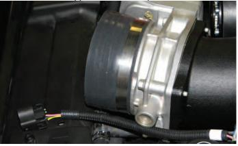
196. Use a 3/32" Allen tool and bolts supplied in Bag #5 to install the supplied MAF sensor in the new inlet tube.
