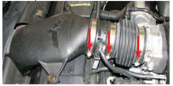
18. Pull out the splash shield above the air filter housings then release the four clamps retaining the air box lids and remove them along with the filters.
