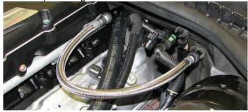
173. Connect fuel injector electrical connectors.
