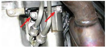
80. Disconnect electrical connector at top of starter.
