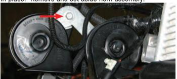
117. Use a 10mm socket to remove the nuts holding the horns to the bracket. Then use a small flat blade screwdriver to remove the wire harness connecting the horns and swap the connectors from horn to horn.
