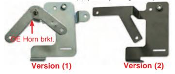
128. **NOTE:** This step only applies to customers who received version (1) of the water pump brackets. Install the supplied stand-off and lock nut onto the OE horn bracket. Proceed by mounting that assembly, with the supplied M6 x 10mm bolt, to the water pump bracket as shown below.
