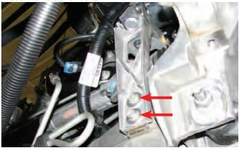
72. Use an 18mm socket to remove the two steering rack nuts and bolts.
