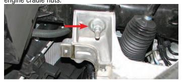
68. Disconnect the ride height sensor electrical connector from each side, if equipped.
