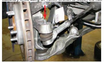
60. Use GM Ball Joint Separator #J 42188 to separate the steering knuckle from the tie rod ball stud then remove the tool and the nut. Use this procedure for both sides.
