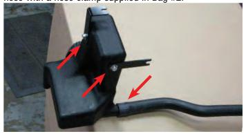
144. Use a 10mm socket to install the brackets supplied in Bag #2 on the reservoir. The image above shows the installed orientation.
