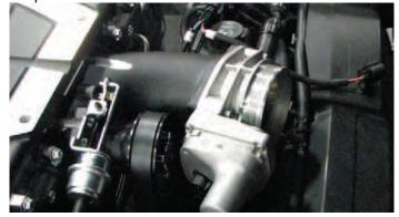
189. Connect ETC harness to the throttle body motor.
