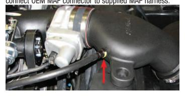
201. Rotate the worm clamps so that the gears are on the driver side then secure the air inlet tube by tightening the worm clamps on the air filter and the silicone hose.
