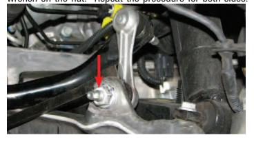
64. Place a catch pan below the steering gear then use an 18mm line wrench to disconnect the two power steering lines from the steering gear.
