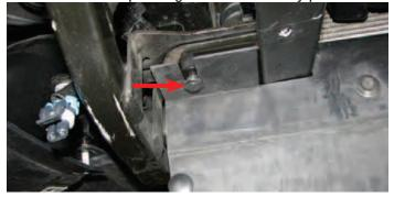
127. Use a 10mm socket to install the pump bracket using the M6 x 45mm bolt and M6 nut on top and the M8 x 30mm bolt on the bottom, all supplied in Bag #2.
