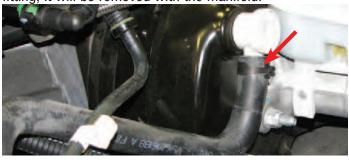
35. Disconnect and remove the two EVAP tubes located at the front of the manifold.
