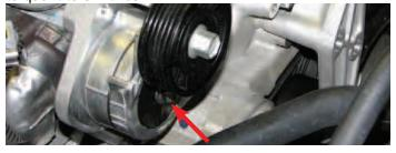
113. Use a 12mm socket and a 20mm bolt supplied in Bag #1 to mount the EVAP purge solenoid on the back of the new tensioner bracket.
