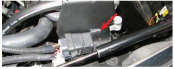
132. Route the intercooler water pump wire harness extending from the relay down to the intercooler water pump and plug in the connector.
