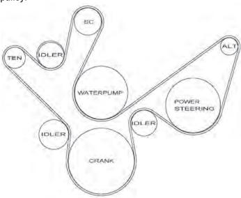
187 Use a breaker bar and a 16mm socket to push the tensioner enough to get the belt on, then double check the routing.
