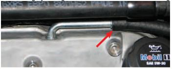
171. Install the supplied driver side PCV hose to the 90° fitting below the air inlet on the supercharger.
