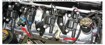
179. Remove the grommets from the stock coil covers.
