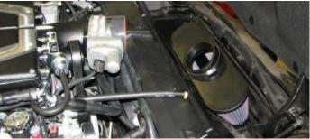
195. Use a T20 Torx driver to remove the MAF sensor from the stock airbox.
