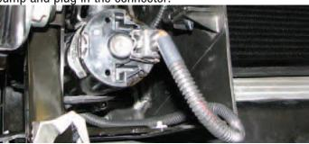
133. Plug the male connector on the T-segment of the harness into the EVAP solenoid then plug the factory EVAP connector into the female connector on the T-segment.
