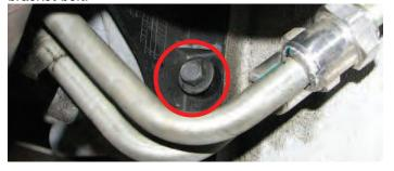
79. Use a 13mm socket to remove the two starter bolts.
