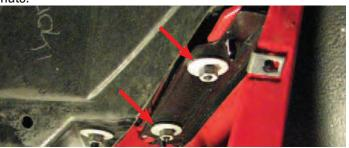
11. Remove the five 7mm and two 10mm nuts retaining the fascia from below.
