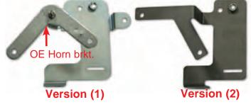
126. **NOTE:** This step only applies to customers who received version (1) of the water pump brackets. Install the supplied stand-off and lock nut onto the OE horn bracket. Proceed by mounting that assembly, with the supplied M6 x 10mm bolt, to the water pump bracket as shown below.
