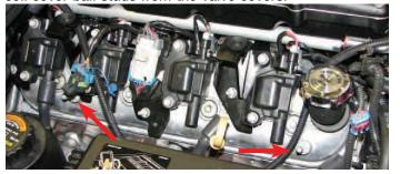
176. Remove the grommets from the stock coil covers.
