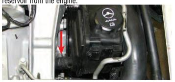
115. Slide the old bracket off the reservoir then install the supplied bracket using a 15mm socket and the stock bolts. Slide the power steering reservoir onto the new bracket and reattach the lower reservoir to pump hose.
