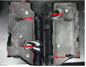
177. Install the stock grommets into the coil cover brackets supplied in Bag #6.
