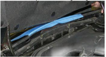
14. The sides of the fascia can be pulled away from the clips holding it in place, then down off the studs. The center section must be pulled up and over the nose section, and the whole assembly pulled straight off and set aside.
