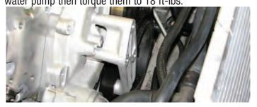
109. Use a 15mm socket and the two stock bolts to mount the new tensioner bracket onto the water pump then torque them to 37 ft-lbs.
