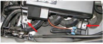
140. Use a 7mm socket to remove the fuse box bolt located in the passenger side fender well.
