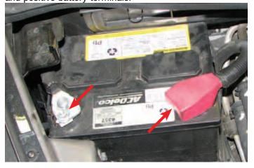
3. Use a 13mm socket and an extension bar to loosen and remove the battery hold down.
