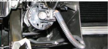
131. Plug the male connector on the T-segment of the harness into the EVAP solenoid then plug the factory EVAP connector into the female connector on the T-segment.
