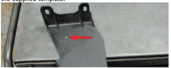
129. Use a 10mm socket and the four stock bolts to reinstall the upper radiator shroud then attach the relay off the supplied water pump wire harness to the upper radiator shroud using the supplied body pin. Open and close the hood to verify the relay clears the hood strut.
