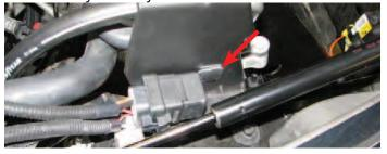
130. Route the intercooler water pump wire harness extending from the relay down to the intercooler water pump and plug in the connector.
