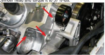
111. Apply blue loctite to the threads of a 20mm bolt supplied in Bag #1, then use a 12mm socket and the supplied washer to mount the pulley on the tensioner bracket and torque it to 18 ft-lbs.
