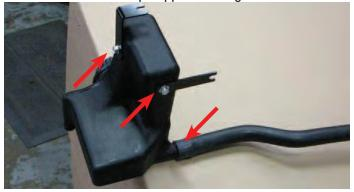
142. Use a 10mm socket to install the brackets supplied in Bag #2 on the reservoir. The image above shows the installed orientation.
