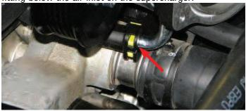
169. Install the supplied fuel line from the firewall fitting to the U-shaped fitting on the driver side fuel rail.
