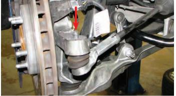
60. Use GM Ball Joint Separator #J 42188 to separate the steering knuckle from the tie rod ball stud then remove the tool and the nut. Use this procedure for both sides.
