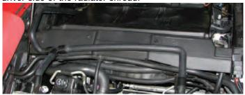
136. Connect the heat exchanger hose assembly to the heat exchanger through the hole drilled in the shroud. Secure the fitting with a hose clamp supplied in Bag #2.
