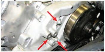
108. Use a 6mm Allen tool and the three 90mm bolts supplied in Bag #1 to install the lower idler bracket on the water pump then torque them to 18 ft-lbs.
