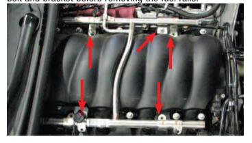
29. Lift the injectors out of the manifold and work the rails forward until they can be set aside.
