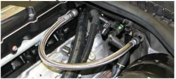
170. Connect fuel injector electrical connectors.
