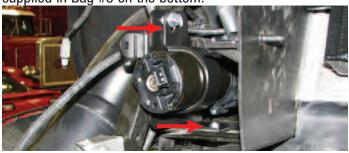
NOTE: There are two different water pump brackets: Version (1) requires the use of your OE horn bracket. Version (2) has an integrated horn bracket. You should have received one of the two brackets; If your supercharger kit includes bracket version (2), you may disregard Step 126.
