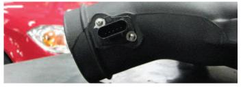
194. Route the supplied MAF wire harness near the driver side of the throttle body.
