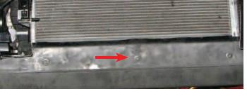
Disconnect horn electrical connector then use a 10mm socket to remove the bolt holding the horn bracket in place. Remove and set aside horn assembly.
