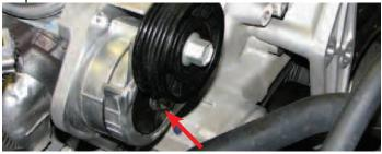
113. Use a 12mm socket and a 20mm bolt supplied in Bag #1 to mount the EVAP purge solenoid on the back of the new tensioner bracket.
