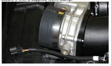
189. Install the grommet supplied in Bag #5 into the new air inlet tube.
