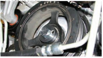
86. Use a 24 mm socket to install the supplied bolt and reamer guide to the end of the crank.
