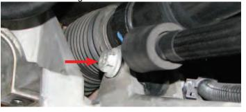
74. Loosen the rear engine cradle nuts with a 21mm deep socket and lower them until there is a gap of 10mm from the cradle to the top of the nut.
