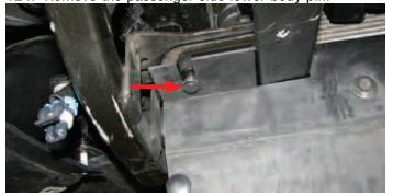
125. Use a 10mm socket to install the water pump bracket using the stock horn bracket bolt on top and the bolt supplied in Bag #3 on the bottom.
