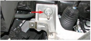
68. Disconnect the ride height sensor electrical connector from each side, if equipped.
