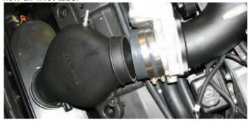
196. Slide the nose of the air inlet tube into the air filter then hold the grommets in place with a socket as you tilt the air inlet tube down into the silicone tube and onto the locator pins.
