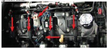
24. Use a 10mm socket to remove the five bolts retaining the coil bracket on each valve cover then remove both coil bracket assemblies.
