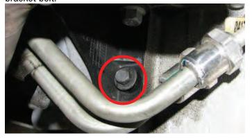
79. Use a 13mm socket to remove the two starter bolts.
