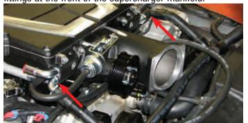
167. Install the passenger side PCV hose on the valve cover fitting by clipping it on. 2008 vehicle owners will need to pull the quick connect fitting out of the supplied hose then slide the hose on the valve cover fitting.
