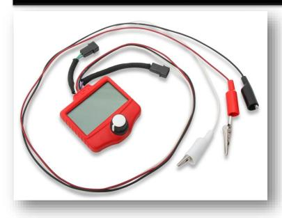
As engine technology changes so does the need for ignition systems and a way to test them. MSD's ignition tester now has the ability to test not only traditional single coil ignition systems but also coil-per-cylinder applications. The 89981 tester even gives you the ability to create an RPM run and let the tester run through the RPM range. This allows you to see the ignition activate any accessories you may be running such as shifters, nitrous solenoids and more.
