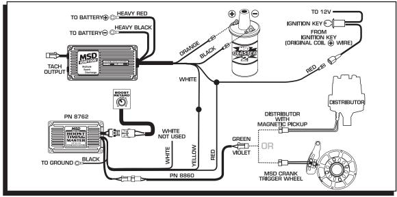
Figure 6 Wiring for MSD 6 Series Using Magnetic Pickup.
