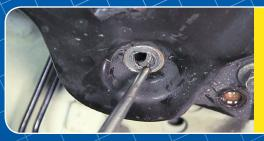
New MOOG design allows technicians to easily align the bushing sleeve to the bolt hole.
