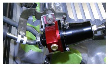
11. It also may be necessary to extend the OEM vacuum/ boost reference line using the enclosed barb union and section of vacuum hose to achieve the desired line routing.
